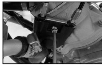
Place the mapping contactor in the "Soft" position (toward the left) and place the motorcycle contact switch in the ON position.
