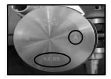
CAUTION: The piston dimension must be measured 10 mm above the apron.
